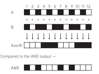
The other outputs in the PERMUTATION SECTION is — CLOCK which outputs a pulse on every step. START which is +5V as long as sequence is running. AND ALL and XOR ALL which preforms the AND function between all patterns and XOR between all patterns (if you set the length of A to 16, B to 15, C to 14, and D to 13 the ALL output will take 43,680 steps to repeat).
