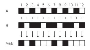
It takes 12 steps for the A and B sequences to repeat (because the lowest common denominator of 3 and 4 is 12). Changing the length of pattern B to 5 instead of 3 makes the sequence 20 steps long. Since  $4 \times 5 = 20$ .
